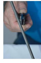
6. Hold the knife straight up and down (like 12:00 and 6:00 on a clock face) as if you are cutting a tomato. Your thumb should be placed on the top or spine of the knife to ensure it is straight up and down.
